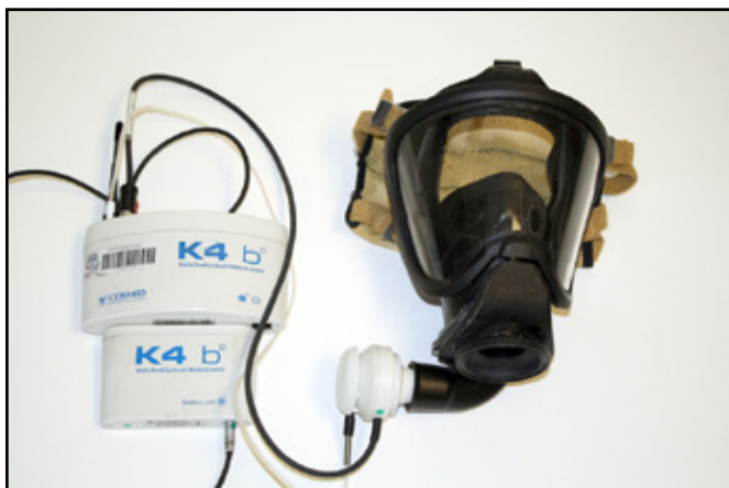
Figure 7. Cosmed K4b2 and custom facepiece used to measure oxygen consumption.
