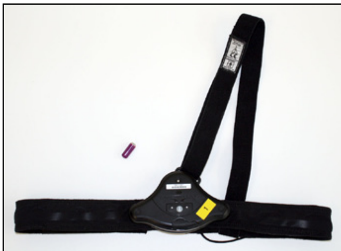
Figure 6. Equivital and cheststrap with core temperature pill.
