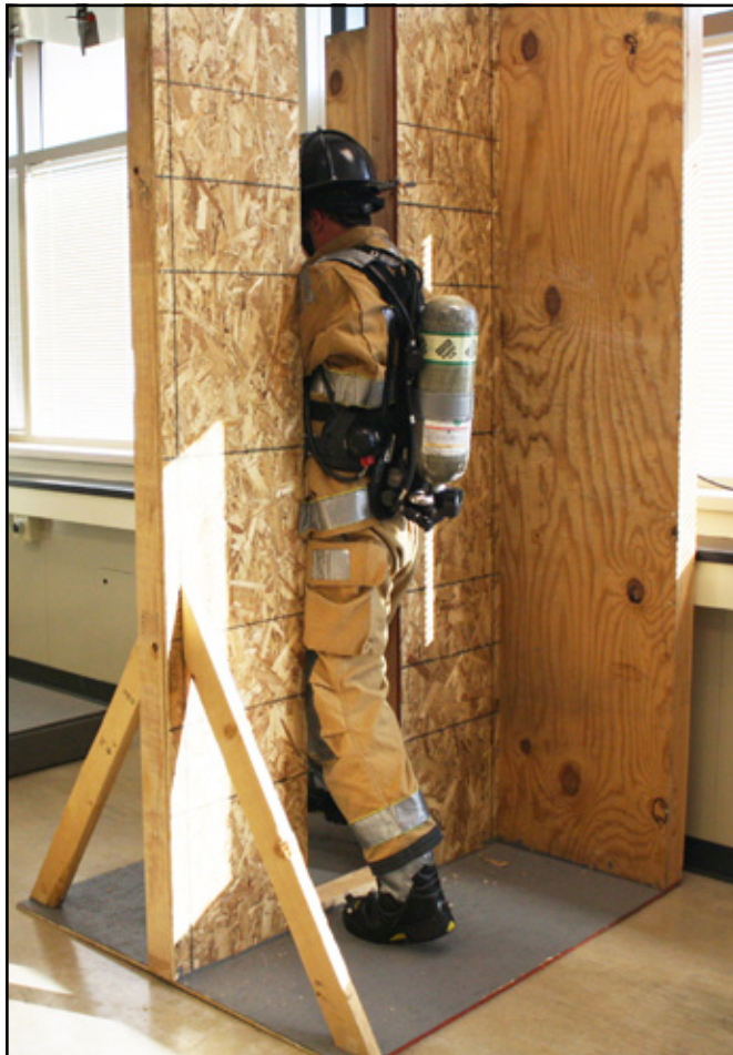
Figure 14. Firefighter passing through stud space.
